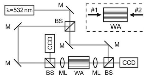
Fig. 1. Experimental setup: ML, microscope lenses; M, mirrors; BS, beam splitters; WA, waveguide array; CCD, CCD cameras. Inset: forward- (#1) and backward- (#2) propagating beams.
