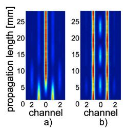
FIG. 5. (Color online) Interaction of in-phase beams for cubic nonlinearity: (a) Fusion of two beams with  $\Delta n_{\rm nl} = 2.8 \times 10^{-5}$ . (b) Nearly independent propagation of two solitonlike beams for  $\Delta n_{\rm nl} = 6.2 \times 10^{-5}$ .
