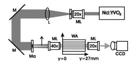
FIG. 1. (Color online) Experimental setup: ML, microscope lenses; L, lens; M, dielectric mirrors; Ma, mask; WA, waveguide array; CCD, CCD camera.
