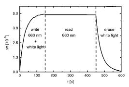
Fig. 1. Refractive-index change for a typical write-readerase cycle. The hologram is recorded with a 660-nm diode laser ( $I_{\rm writing} = 0.65 \text{ W/cm}^2$ ) and white light from a Xe lamp for gating. Nondestructive readout is performed with one of the writing beams, and hologram erasure is possible with the gating light.
