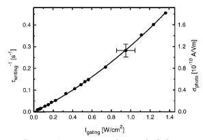
Fig. 4. Inverse time constant  $1/\tau_{\rm writing}$  for hologram writing and photoconductivity  $\sigma_{\rm photo}$  versus gating intensity at 488 nm. The curve is a fit according to  $\sigma_{\rm photo} = aI_{\rm gating} + bI_{\rm gating}^2$ , where *a* and *b* represent fit parameters.
