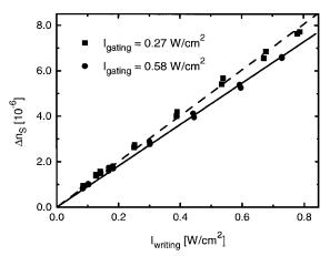
Fig. 3. Saturation values  $\Delta n_S$  of refractive-index changes as a function of the writing intensity  $I_{\rm writing}$  for two different gating intensities. The lines are linear fits to the measured values.
