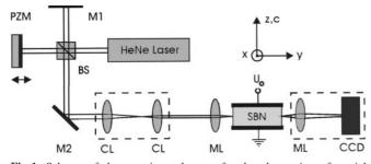
**Fig. 1.** Scheme of the experimental setup for the observation of spatial soliton interaction in the planar waveguide. M1, M2, mirrors; BS, beam splitter; PZM, piezo-mounted mirror; CLs, cylindrical lenses; MLs, microscope lenses;  $U_0$ , externally applied high voltage; SBN, SBN waveguide; CCD, CCD camera
