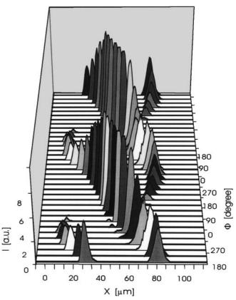
**Fig. 2.** Intensity distribution I(x) on the endface of the planar SBN waveguide as a function of the relative phase  $\Phi$  of two solitons that intersect at an angle  $2\Theta \approx 1.4^{\circ}$  inside the sample. The input power of each soliton is  $3 \,\mu$ W and the soliton width (FWHM) is about  $8 \,\mu$ m
