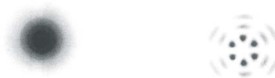
Figure 8.1-7 Distributions of the intensity of the (a) LP_{01} and (b) LP_{34} modes in the transverse plane, assuming an azimuthal \cos l\phi dependence. The fundamental LP_{01} mode has a distribution similar to that of the Gaussian beam discussed in Chap. 3.
