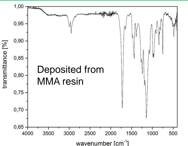
MMA resin application: thicker coatings with low loss of monomer
