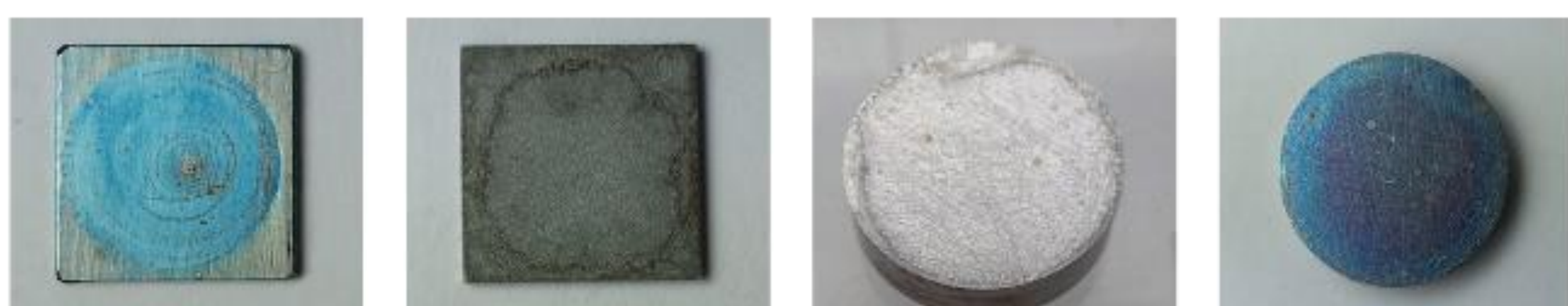
heated polycarbonate layer on iron foil heated polycarbonate layer on chromium foil unheated polycarbonate layer on steel sample heated polycarbonate layer on steel sample
