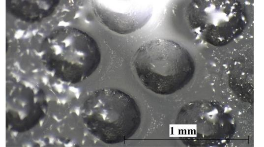
Surface of polymerized film after plasma treatment:
