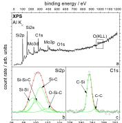
102 284 288 293 100 10 276 280 binding energy / eV binding energy / e\ XPS survey and detail spectra
