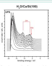
After the preparation of a monoatomic layer of Calcium, a dosage of 14L  $H_2O$  was sufficient to lead to a saturated hydroxide. No oxidic structures visible in MIES nor UPS. The oxidic part (I) of the O1s feature is assumed to originate from the substrate
