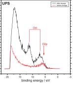
Having prepared another monolayer of Calcium upon the monomolecular film of Calcium hydroxide, spectra of MIES and UPS before and after the evaporation show a significant reduction of the surface according to  $Ca(OH)_2 + Ca \rightarrow 2CaO + H_2$
