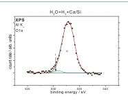
The evaporation of Calcium in an atmosphere combined of  $1.10^{-7}$  mbar H<sub>2</sub>O and  $9.10^{-7}$  mbar H<sub>2</sub> leads to a clean film of Calcium hydroxide due to MIES, whe reas UPS shows a small amount of oxide intensity. The XPS results point out a fraction of less than 3% oxide (I) besides the hydroxide (II).
