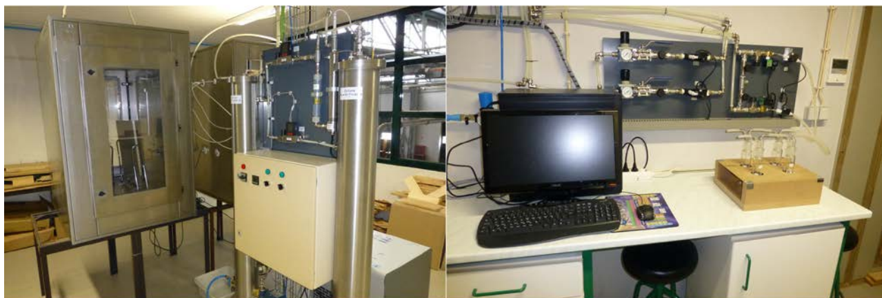
Figure 1: Apparatus of a chamber method (EN 717-1), including the chamber and air source (left) and collecting system (right).
