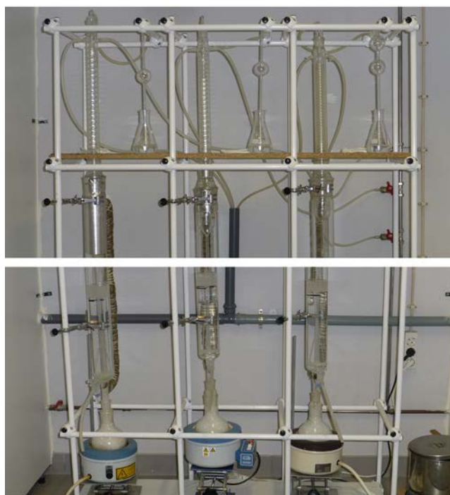
Figure 4: Perforator equipment used in EN 120 (lower image shows the boiling of test samples in toluene, and upper image shows collecting of resulting formaldehyde dissolved in water).
