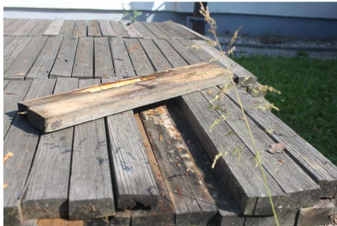
Figure 2: Development of the fungal mycelia on the control specimens. Please note darkening as the sign of severe degradation of the wood.
