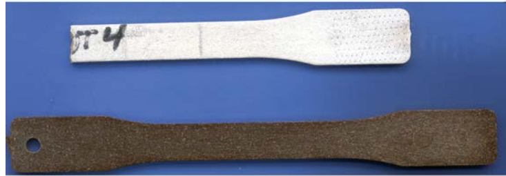
Figure 6: Wood-thermoplastic composite before (lower) and after (upper) one year exposed outdoors.
