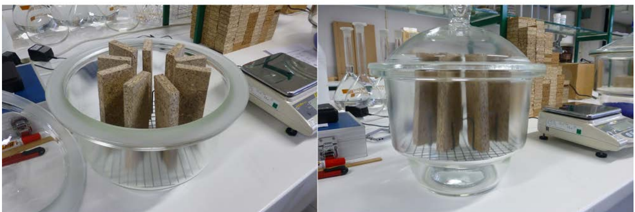
Figure 3: Apparatus of desiccator testing, according to JIS A 1460 (on left, an open desiccator with test pieces and an example of a test running, at right).
