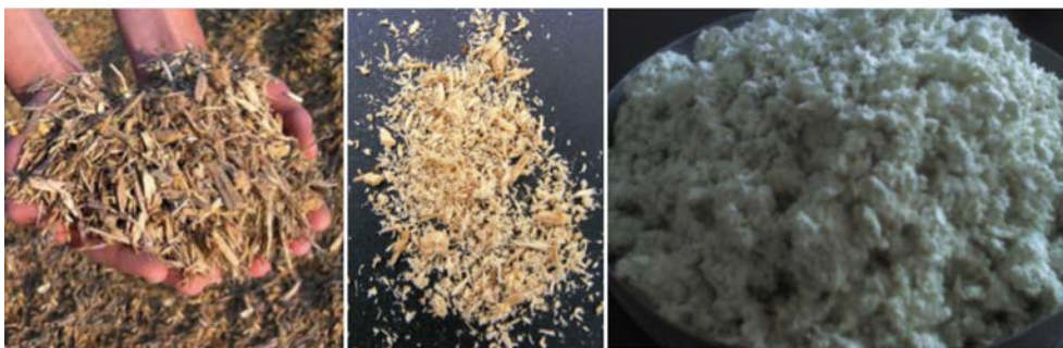
Figure 2: Forest residues chipped and hammer milled into particles and fibers.
