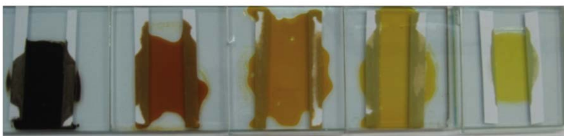
Figure 2: Colour change of liquefied wood during manganese sulphate/sodium bicarbonate activated hydrogen peroxide oxidation as a function of the quantity of hydrogen peroxide applied (from right to left: 0 %, 20 %, 40 %, 60 % and 80 % of H_2O_2 ).
