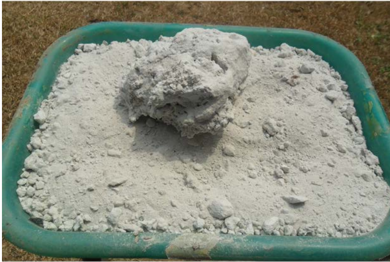
Figure 2: Welders' carbide waste.
