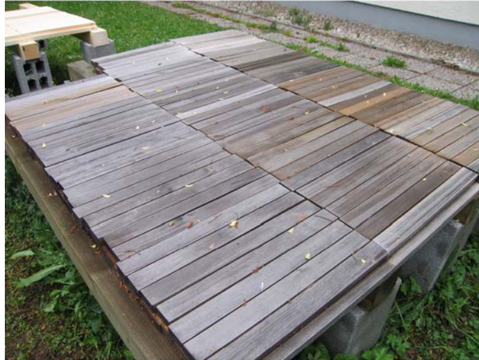
Figure 1: Test set up of the specimens exposed in use class 3 conditions according to the double layer test method after one year of exposure.
