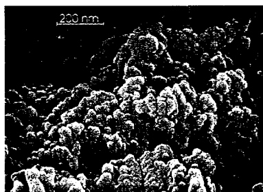
Fig. 6. High Resolution Scanning Electron Microscopy (HRSEM) image of the nanoscale silicon.
