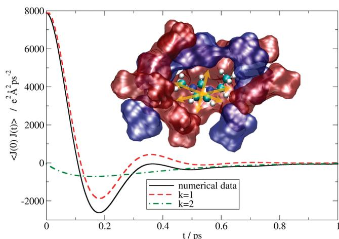
**Figure 9:** Current autocorrelation function  $\langle J(0)J(t) \rangle$  and its decomposition into two damped oscillator functions. The frequency  $\omega_1$  of the red oscillator function corresponds to far IR measurements.
